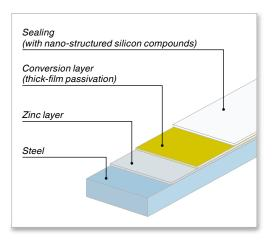
Fittings manufactured from steel or die-cast zinc are galvanised, passivated and sealed. Thick-layer passivation and sealing serves to improve the corrosion resistance and the appearance of zinc coatings on metal.
