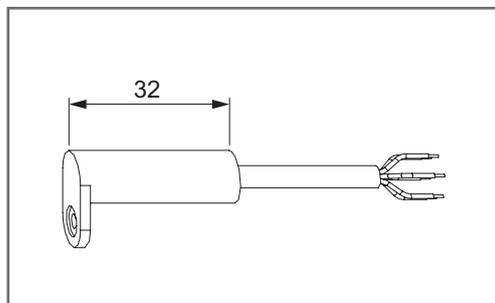
*Magnetic switch for combined opening and locking monitoring*
