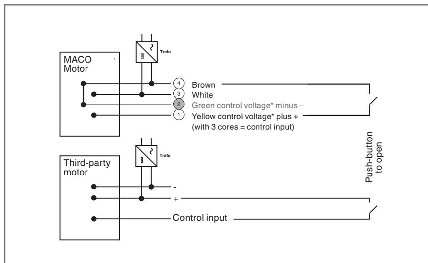
*Comparison MACO motor (when used with only 3 connections) with third-party and positive pole control contact*
