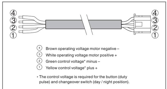
*Connection cable to the motor*
