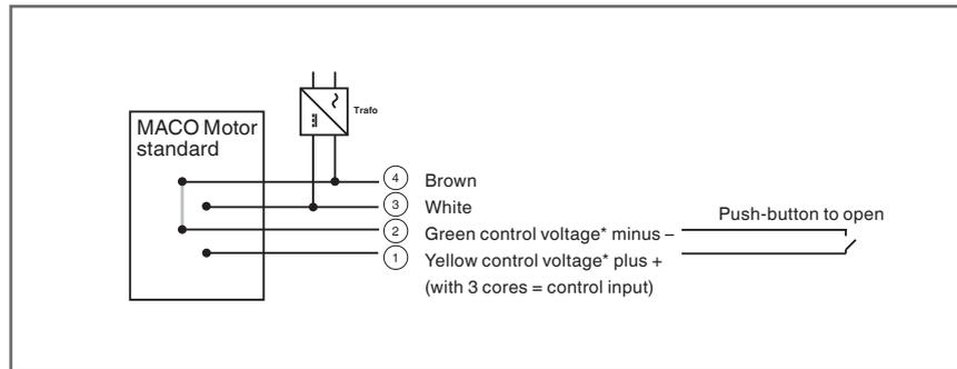
All MACO access controls operate on the above mentioned principle and are therefore designed for the four connections.
