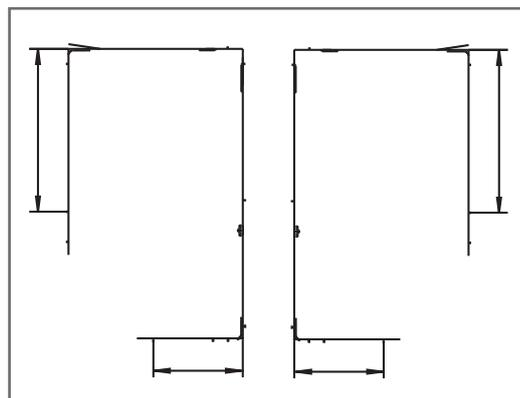
All measured values and the clearance added together give the distance from the frame to the magnetic cam. To determine the cable bore for the reed contact closing part, 39 mm should be added to this value if on the hinge-side and 39 mm should be subtracted if on the lower horizontal side (due to closure directions). The mounting holes are 11 and 29 mm away from the connection cable hole.
