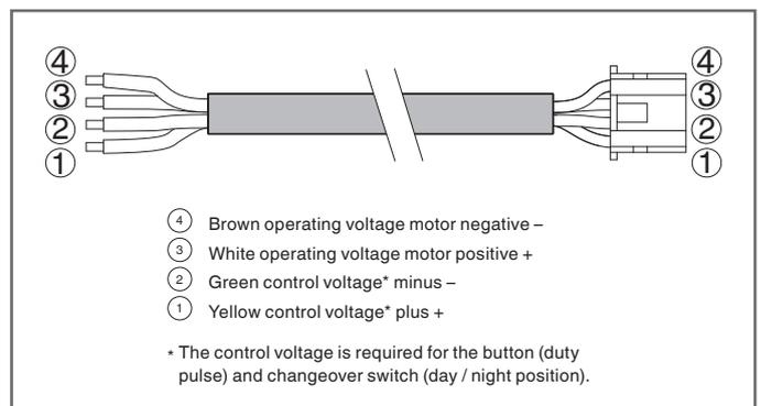
*Connection cable to the motor*
