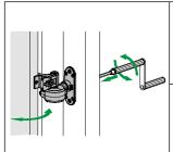
Open and fix the shutter - insert the crank and rotate to open the shutter.
