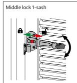
Lock the shutter in its closed position.
