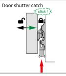
Fix shutter in open position. Swing the shutter backwards until it audibly snaps in. Shutter is thereby fixed.
