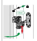
Fix shutter in open position. Swing the shutter backwards until it audibly snaps in. Shutter is thereby fixed.
