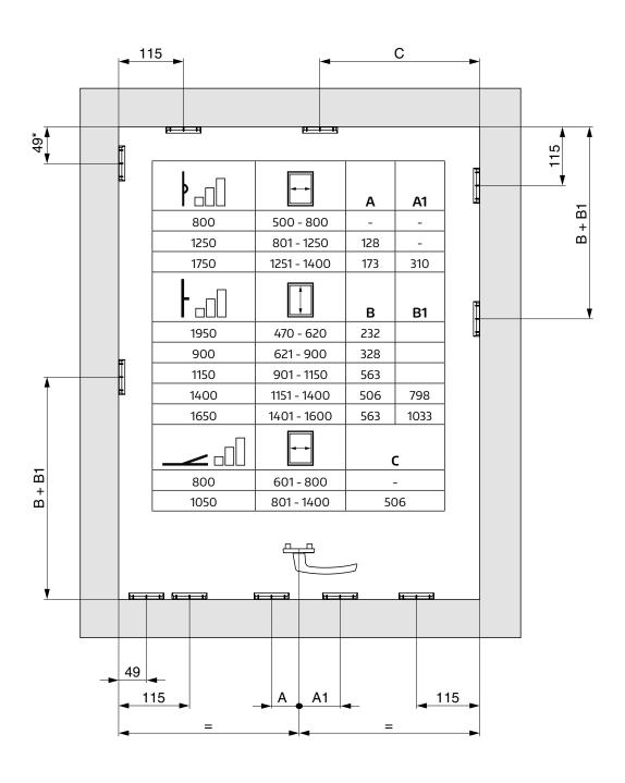
$<sup>^{\</sup>ast}$  only when using short corner element with 1 i.S.
