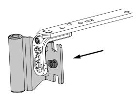
2. Turn the bayonet bolt with TX20 order no. 40680 in the direction of the arrow.
