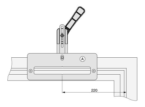
Position the routing jig  $\bigcirc$  Art. No. 214756 asdepicted and rout with  $\emptyset$  8 mm routing cutter and  $\emptyset$  27 mm guide ring.
