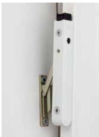
When setting down the window sash on turn-only and tilt-and-turn windows gradually, the MULTI-Vent tilt restrictor allows you to select the opening angle freely. The integrated braking effect means that the sash stops at the desired width without latching.
