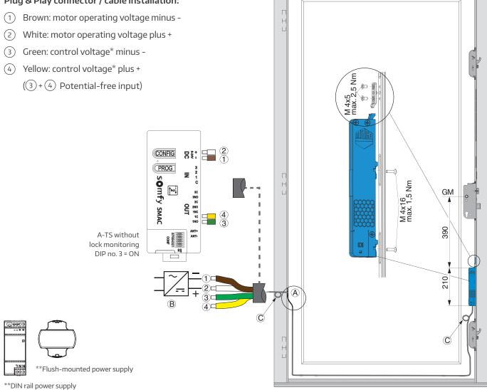
\*\*It is recommended to use the A-TS for motorised opening only with the power supply units that have been tested and approved for this purpose. These are designed for an input voltage of 220-240 V / 50-60 Hz and provide an output voltage of 24 V DC 1A with dynamic overcurrent 3A for 500 ms/ 7A for 100 ms. Alternatively, third-party products must have an output voltage of 12 - 24 V DC with min. 1.5A.
