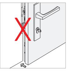
Do not lock the locking bar when the door is open!
