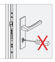
Only close the lock with the corresponding operating key!
