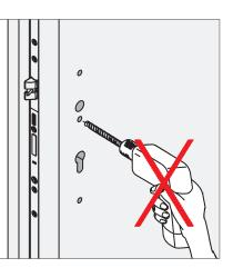
Drill all holes before installation of the lock.
