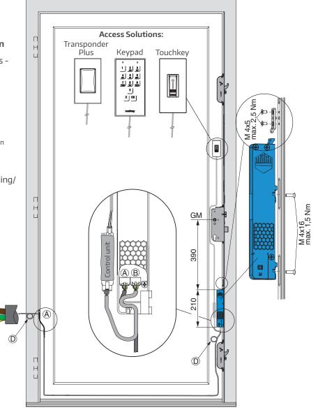
\*\*It is recommended to use the A-TS for motorised opening only with the power supply units that have been tested and approved for this purpose. These are designed for an input voltage of 220-240 V / 50-60 Hz and provide an output voltage of 24 V DC 1A with dynamic overcurrent 3A for 500 ms/ 7A for 100 ms. Alternatively, third-party products must have an output voltage of 12 - 24 V DC with min. 1.5A.
