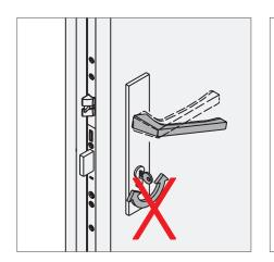
Do not simultaneously press the handle and turn the key!
