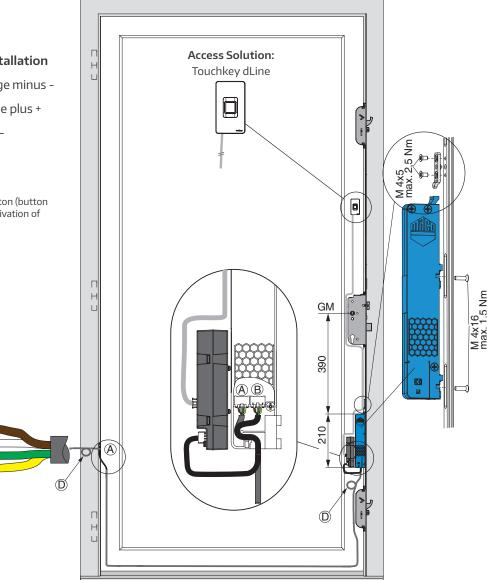
\*\*It is recommended to use the A-TS for motorised opening only with the power supply units that have been tested and approved for this purpose. These are designed for an input voltage of 220-240 V / 50-60 Hz and provide an output voltage of 24 V DC 1A with dynamic overcurrent 3A for 500 ms/ 7A for 100 ms. Alternatively, third-party products must have an output voltage of 12 - 24 V DC with min. 1.5A.
