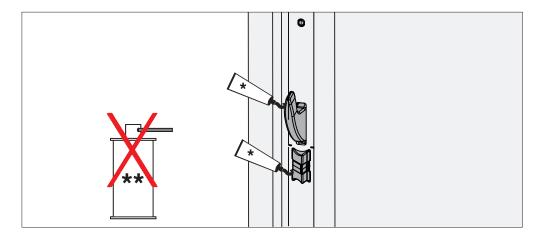
Lubricate the MF-HO locking element 1x annually!
