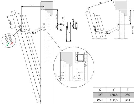
(A) Screws as long as possible, at least Ø 4x45 mm. In the case of PVC profiles, the threaded connection must go through the reinforcement.
