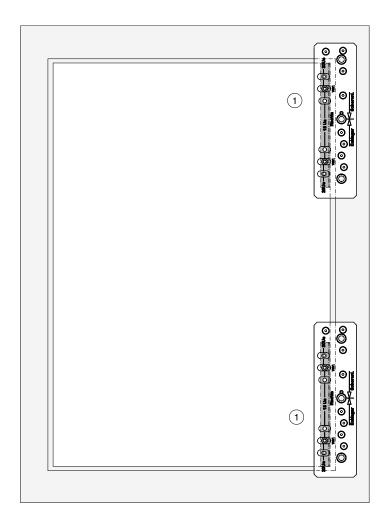
① Insert drilling jig for right sash Item No. 213096 or for left sash Item No. 213097 in frame rebate corners at the top and bottom (with air gap 12 mm) and pre-drill with  $\emptyset$  3 or  $\emptyset$  9 mm drill.
