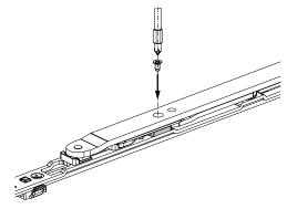
4. Screw the anti-slam device/scissor stay restrictor in place.
