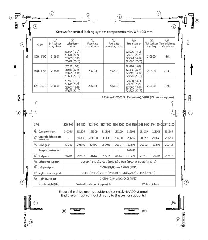
Fit the handle (handle position vertically upwards = locked position) and tear through both central locking systems in direction horizontal handle position (= tilted position).
