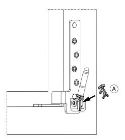
1. Attach the insertion tool A to pivot post pin and hinge the sash at a 90° opening angle in the pivot post.
