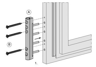
1. Insert the Corner Support  $^{\textcircled{A}}$  in the holes and screw tight with the three, longest possible screws  $^{\textcircled{B}}$ .
