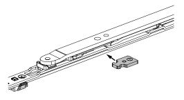
3. Insert the anti-slam device light (Item No. 368076) or scissor stay restrictor (Item No. 368077).
