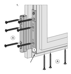
1. Place the rebated corner support in the Eurogroove and screw tightly into place with nine screws A at least O 4 x 25 mm .
