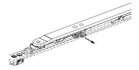
2. Pull the anti-slam device heavy (Item No. 368075 = delivery state) out laterally.
