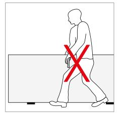
The multi-point lock must be replaced as soon as traces of use of force are visible! Do not carry the door leaf with the handle!
