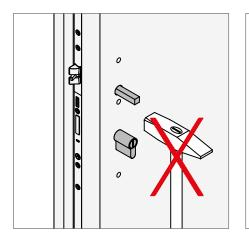
Do not force the handle pin through the lock nut!
