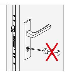
Only close the lock with the corresponding operating key!
