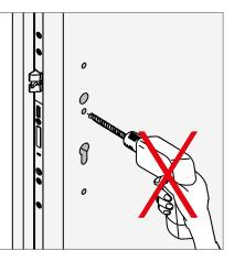
Drill all holes before installation of the lock.
