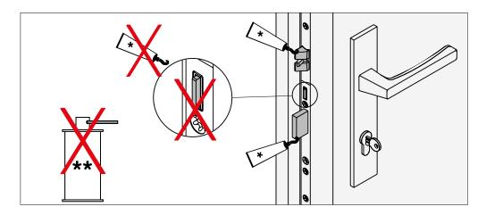
The door lock (lock case) is delivered with an intensive lubrication of high-performance greases and must NOT be relubricated!
