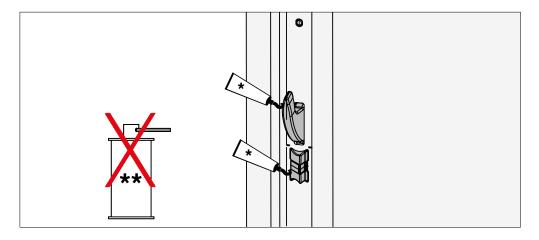
Lubricate the MF-HO locking element 1x annually!
