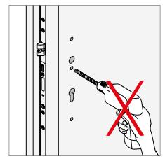
Drill all holes before installation of the lock.
