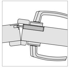
Double-sash doors must not be forced over the inactive leaf!
