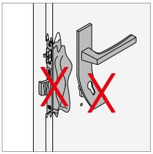
The multi-point lock must be replaced as soon as traces of use of force are visible!
