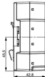
Mounting on a standard profile rail DIN EN 60715-TH35-15/7,5 is possible. Alternatively, the device can also be mounted in flush-mounted box. Therefore, the mounting clamp on the back of the device can be removed by loosening the two screws.
