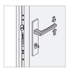
Only apply load to the handle in the normal direction! Apply a maximum force of 15 kg in the direction of actuation (on the handle).
