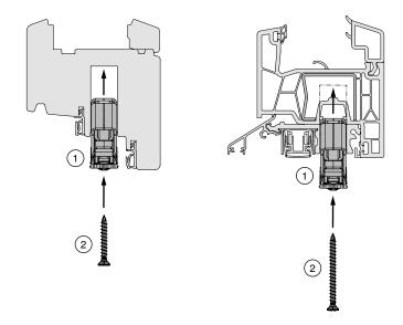
Slide VCI-wrapper item no. 371808 over hook lock housing (see note). Insert locking hook 1 in routing and screw in place. Screw dimension 2, in PVC the screw must protrude through both fitting grooves. Screw diameter min. 4 x 35 mm.
