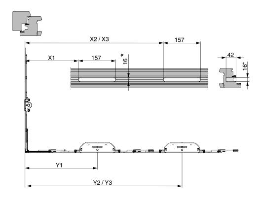
\*Routing with milling cutter Ø 16 at least 42 mm in sash (fitting groove centre).
