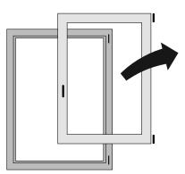
The casement door sash is hinged in the frame according to the assembly instructions of the hinge-side used.
