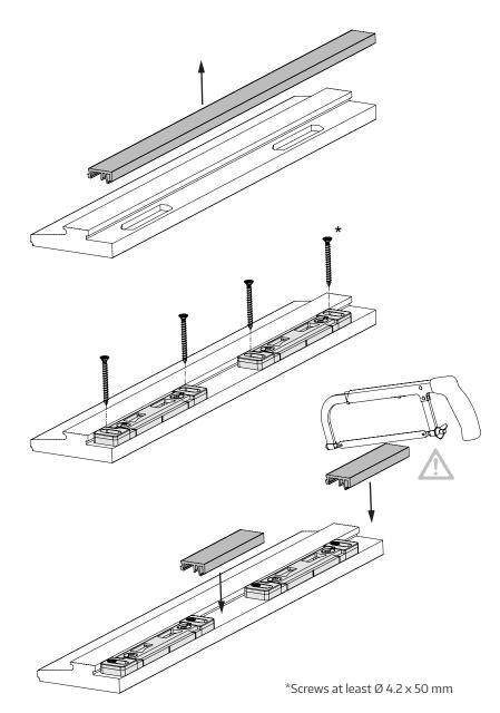
Threshold with frame must be fully lined. The load must be borne in the lining profile / substructure. Country-specific specifications and guidelines for the floor structure must be taken into account.
