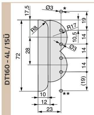
Drilling depth of the DT drill hole 8 mm.
