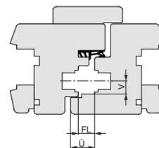
Possible values for air gap, rebate depth, offset and rebate leg:
