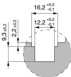
French window sash with aluminium groove
