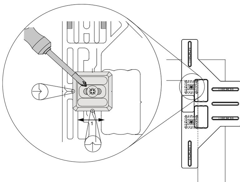
Remove the DT130 pre-mounted stop pieces (Art. No. 41862) and fit the DT160 stop pieces (Art. No. 370313). Adjust the notches ① to the profile used. Fix the stop pieces in place.
