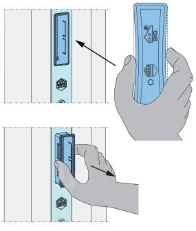
1 Press the existing routing cover together as shown in the graphic to release the retaining tabs from their recess. Now, pull the routing cover straight out.
