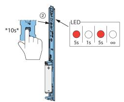
2 Press and hold the user button for at least 10 seconds. After about 5 seconds, the status LED will briefly turn off and then light up again. Keep holding the button until the LED turns off completely. Release the user button to perform the hard reset.
