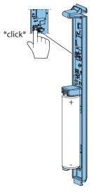
Briefly press the user button. This process can be repeated at any time if required.
