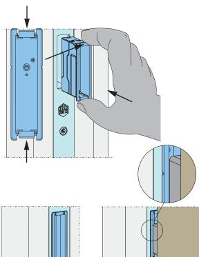
2 Take product ① and press the tabs at the top and bottom together as shown in the graphic. Slide the sensor into the recess for the routing cover. Note the two different installation options for the sensor that vary depending on the door lock. Ensure that the routing depth is sufficient and that the positioning notches cover the deadbolt of the door lock.
