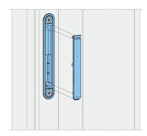
2 Close the housing with the cover and check the mechanical function. Mounting is now complete; all further steps are the responsibility of the end customer.
