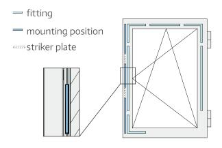
1 Please select a suitable mounting position for the Sense by Maco | Window T&T using the enclosed graphic. Note that mounting must only be carried out on the gear side in positions where there is no cam or striker plate.
