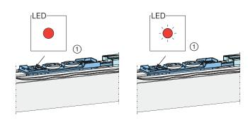
**3** The device will automatically enter pairing mode, indicated by a flashing status LED.
