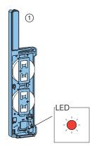
3 Once the hard reset is complete, the product automatically enters pairing mode. This is indicated by a flashing status LED. Continue with the "(Initial) Start-up" chapter.
