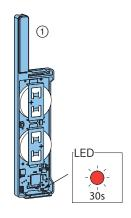
2 The Sensor ① now enters calibration mode for 30 seconds, during which the status LED will flash.
