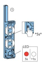
2 Press the user button for at least 5 seconds until the LED briefly turns off. Release the user button to perform the soft reset.
