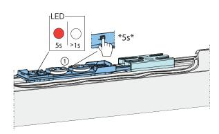
2 Press and hold the user button for at least 5 seconds until the LED shortly turns off. Release the user button to start the soft reset.
