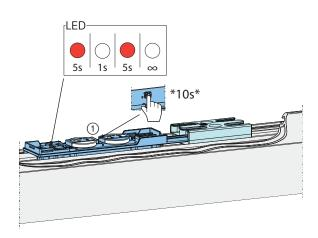
2 Press and hold the user button for at least 10 seconds. After 5 seconds, the status LED will briefly switch off and then lights up again. Continue to push the user button until the LED turns off permanently. Release the user button to start the hard reset.
