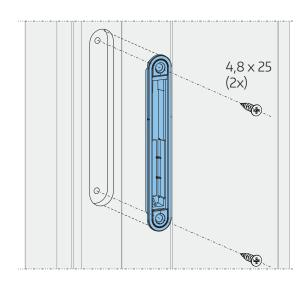
$\bullet$  Screw the housing in place using 4.8 x 25 (2x).
