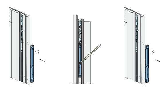
1 Position the housing on the open sash and mark the drill holes.
