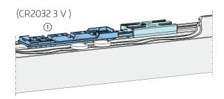
2 For battery replacement: Insert suitable batteries (CR2032, 3 V, not included) and close the housing.
