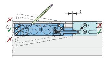
4 Position housing at striker plate as shown and mark two diagonal holes.
