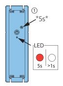
wthe LED shortly turns off. Release the user button to start the soft reset.
