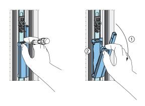
① Open the housing. To do this, use a flat object (e.g., a screwdriver) to push the housing tab upwards and carefully pull at the recess. Depending on the mounting position, remove either sensor ① or the housing cover ②.
