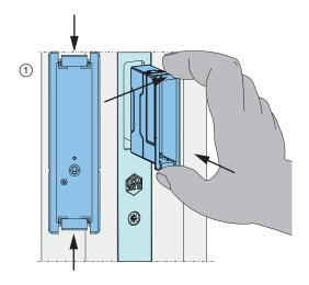
2 Rotate sensor ① by 180° and squeeze the tabs at the top and bottom as shown in the graphic. Slide it back into the recess. Ensure that the positioning notches are level with the deadbolt of the door lock. Check the mechanical function of the door. Mounting is now complete. All further steps will be carried out by the end customer.
