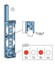
2 Press the user button for at least 10 seconds. After approx. 5 seconds, the status LED will briefly turn off and then light up again. Continue to hold the user button until the LED turns off permanently. Release the user button to perform the hard reset.
