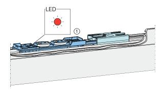
3 Once the hard reset is completed, the product will automatically enter pairing mode. This is indicated by a flashing status LED. Continue with step 4 in chapter "Start-up".
