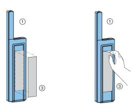
Semove the protective film from the other side of adhesive tape (5).
