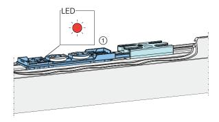
3 Once the soft reset is completed, the product will automatically enter pairing mode. This is indicated by a flashing status LED. Continue with step 4 in chapter "Start-up". Recalibration (see chapter "Calibration") is possible, but not necessary.
