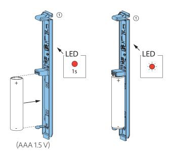
2 For battery replacement: Insert a suitable AAA battery (1.5 V, not included) and close the housing.
