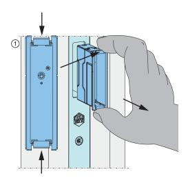
1 To make pressing the user button easier, carefully release the sensor by pressing in the tabs at the top and bottom of the housing and pull it out if necessary.
