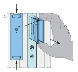
1 Carefully release the sensor by pressing in the tabs at the top and bottom of the housing, and then pull it out. Note the current installation position and lateral positioning notches.
