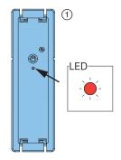
3 Once the hard reset is completed, the product will automatically enter pairing mode. This is indicated by a flashing status LED. Continue with step 5 in chapter "(Initial) Start-up".
