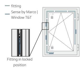
1 Please select a suitable installation position for the Sense by Maco | Window T&T using the graphic provided.
