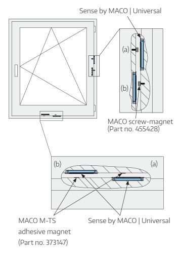
For opening monitoring, the Sense by MACO | Universal can be installed in either the frame (a) or the sash (b), but installation in the sash is recommended if possible.
