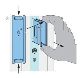
① Carefully press the tabs at the top and bottom of the housing and pull sensor ① out of the recess.
