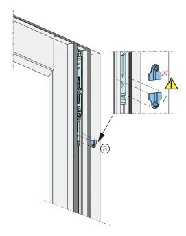
3 Insert magnet holder ③ into the unused hole of the corner drive or the extendable centre lock.
