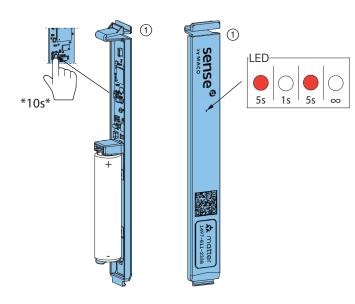
2 Press and hold the user button for at least 10 seconds. After about 5 seconds, the status LED will briefly turn off and then light up again. Keep holding the button until the LED turns off completely. Release the user button to perform the hard reset.
