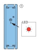
automatically enter pairing mode. This is indicated by a flashing status LED. Continue with step 5 in chapter "Start-up". Recalibration (see chapter "Calibration") is possible, but not necessary.
