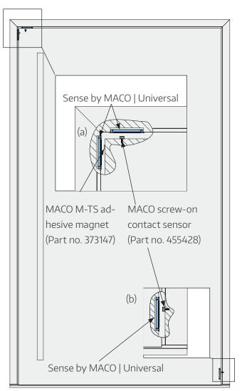
For opening monitoring, Sense by MACO | Universal can be installed in either the door frame (a) or the door leaf (b).
