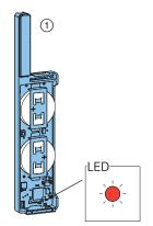
3 Once the soft reset is complete, the product automatically enters pairing mode. This is indicated by a flashing status LED. Continue with the "(Initial) Start-up" chapter. A renewed calibration (see chapter "Calibration") is possible, but not strictly necessary.
