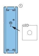
4 Re-insert the sensor into the component. Pair the sensor with your smart home ecosystem. Refer to the "Integration into the smart home System" guide on page 51 or the instructions provided by your smart home ecosystem supplier. Once pairing is successful, the status LED will turn off. The sensor status will be displayed as "Open" in the app. Proceed with the "Calibration" chapter.
