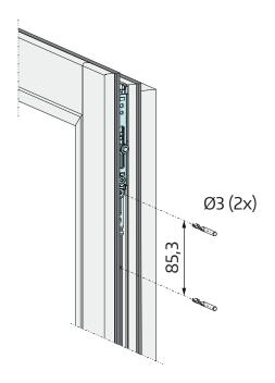
2 Pre-drill the holes using a Ø3 mm drill bit.
