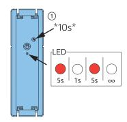
2 Press and hold the user button for at least 10 seconds. After 5 seconds, the status LED will turn off and then lights up again. Continue to push the user button until the LED turns off permanently. Release the user button to start the hard reset.
