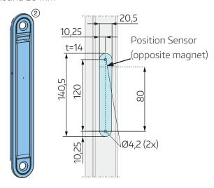
1 Select the appropriate cover plate for the profile system, position the sensor opposite the magnet, and rout the necessary clearance in the frame. Predrill 2x Ø 4.2.
