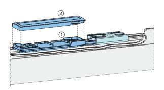
• Close sensor ① with cover ② and check the correct mechanical function of the window. Mounting is now complete. All further steps will be carried out by the end customer.
