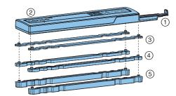
3 Clip the required spacers (③, ④, ⑤) onto sensor ①. Arrange the spacers to create a stable base for the sensor.
