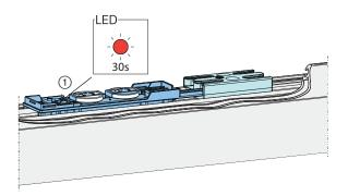
2 The sensor ② will now enter calibration mode for 30 seconds. During this time, the status LED will flash.
