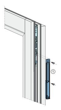
4 Reinsert housing ① into the fitting groove and fasten it using suitable screws (e.g. 4 x 28). Tighten the screws by hand only—do not overtighten.
