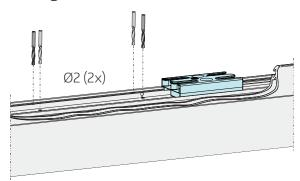
**5** Pre-drill two diagonal holes using a Ø 2 drill bit.
