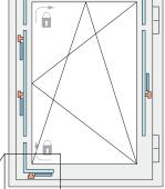
Mount the fitting component or magnetic cam according to the instructions and install the fitting. Determine the closing direction to ensure correct sensor mounting.
