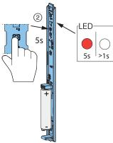
2 Press and hold the user button for at least 5 seconds until the LED briefly turns off. Release the user button to perform the soft reset.
