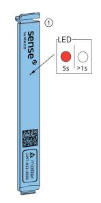
2 Press and hold the user button for at least 5 seconds until the LED briefly turns off. Release the user button to perform the soft reset.
