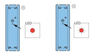
3 The device will automatically enter pairing mode, indicated by the flashing of the status LED. Close the battery compartment.
