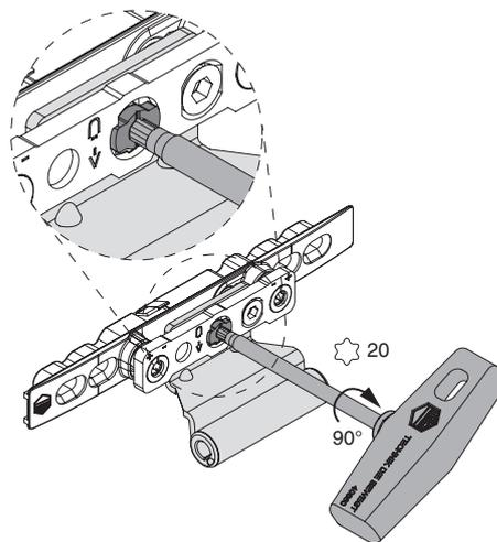
Turn the bayonet coupling with  $\star 20$  (order no. 40680) in the direction of the arrow.
