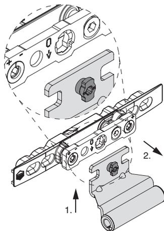
Insert the rebated scissor stay support arm into the tilt-only and turn-only hinge and insert the bayonet coupling from behind through the bayonet opening (ensure correct position).
