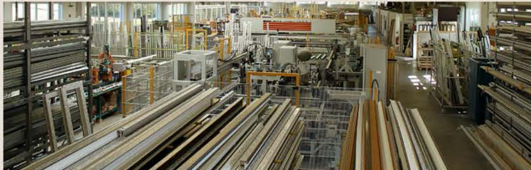
The aluminium shells are manufactured in their own aluminium department, and can be supplied welded on request.
