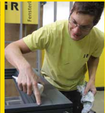
Prior to the painting process, any damage to the timber is rectified or glue residue is removed so that the surface is as smooth as possible.
