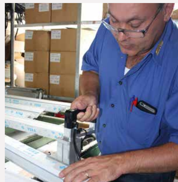
Leo Löffler shows how the punch works that creates the gap in the seal for the installation of the rebate ventilator.
