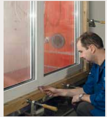
Weather test rig for air and water tightness / wind resistance
