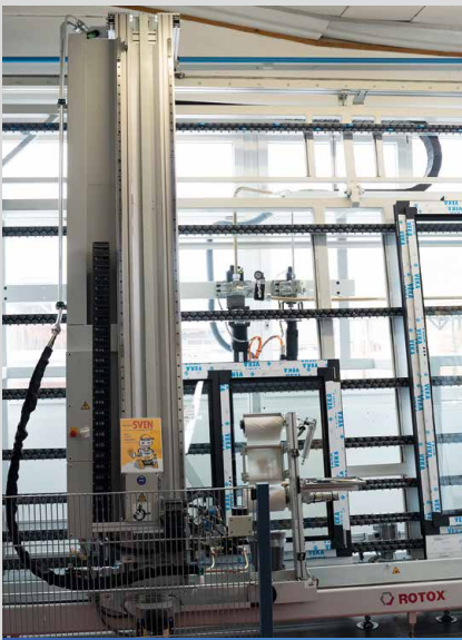
Bonding machine Sven. It detects the size and profile thickness of the element by laser and adjusts itself accordingly.
