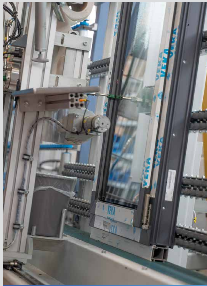
Bonding machine Sven. It detects the size and profile thickness of the element by laser and adjusts itself accordingly.
