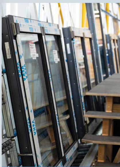
When glass and sash are married to the frame, it goes into the bonding. Windows and French doors on the way to the bonding machine
