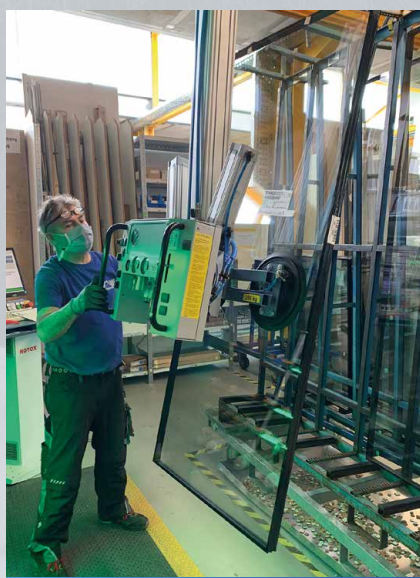
When glass and sash are married to the frame, it goes into the bonding. Windows and French doors on the way to the bonding machine
