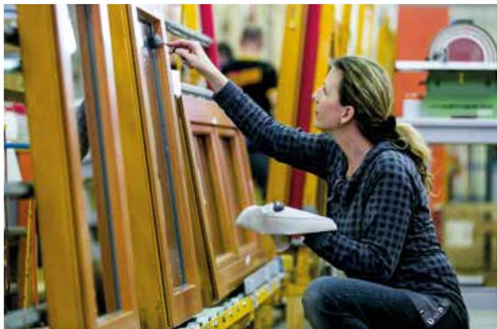
The manual wet sealing with special silicone ensures 100% impermeability.
