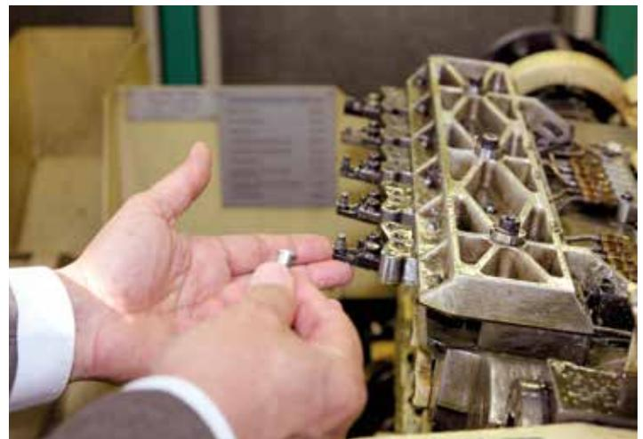
Through the interchangeable insertion of tool slides, cutting dies can be adjusted and changed over within five to ten minutes. The machine moves 1000 kg of steel in half a second, which allows MACO to carry out flexible punching according to customer requirements.
