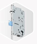
The main latch automatically triggers the locking mechanism as soon as the door enters the frame. In addition, a magnet monitors the correct closing position, forming the two criteria to ensure secure locking. Two hooks and the central deadbolt automatically engage, and the door is triple locked all without a key.
